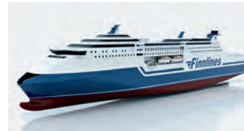
Superstar ro-pax vessels run on traditional fuels and use scrubbers and lithium batteries.
